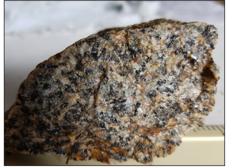
Fig. W11.5 Hand specimen of leucodolerite from Locality 1. The light areas are plagioclase feldspar.
